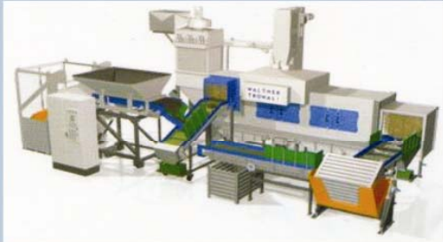
Walther Trowal THM 500/2/E system includes all in picture in like new condition Part size 350mm x 1000mm
