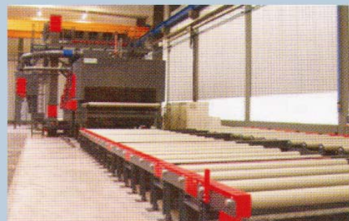
Rosler RDGE roller conveyor machine 1000mm x 400mm opening, conveyor in and out
